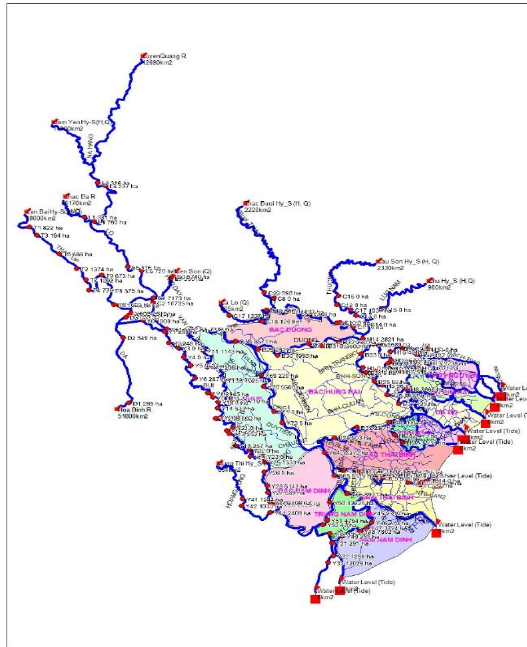
Diagram of Mike 11 model to calculate water level and hydraulic water.
